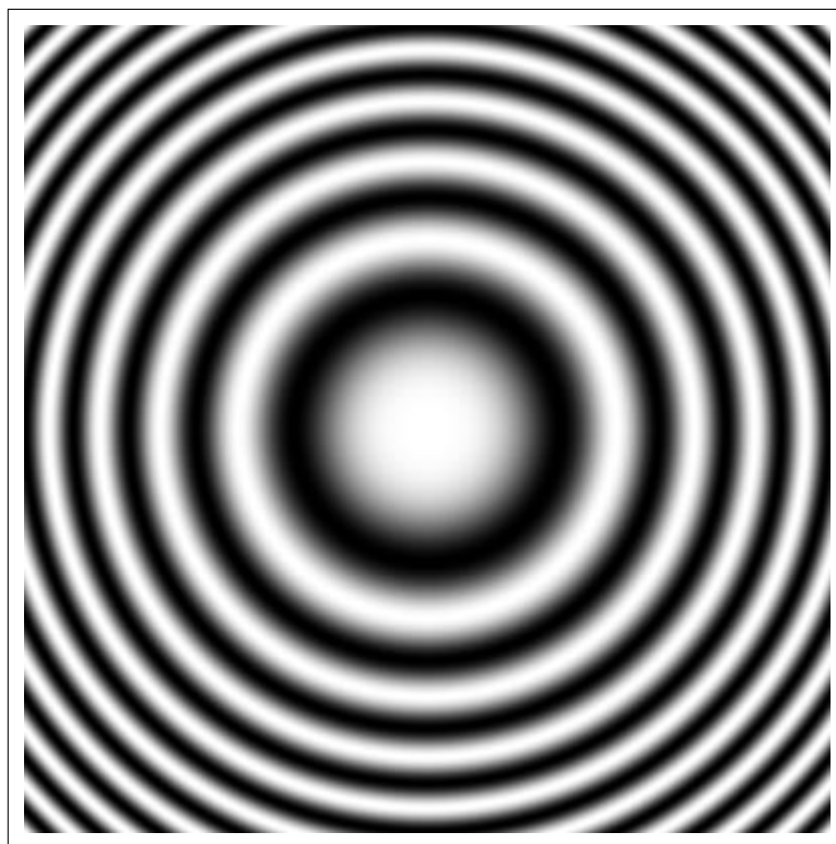
FIGURE 4. Simulated interference pattern in the plane of the diode.
